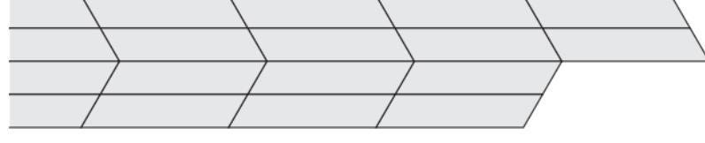
After the installation of three to four rows, adjust again. Use spacers. Make sure these first rows are accurate. Use a marking band or straightedge, etc. Continue with the rest of the room in the described way.
