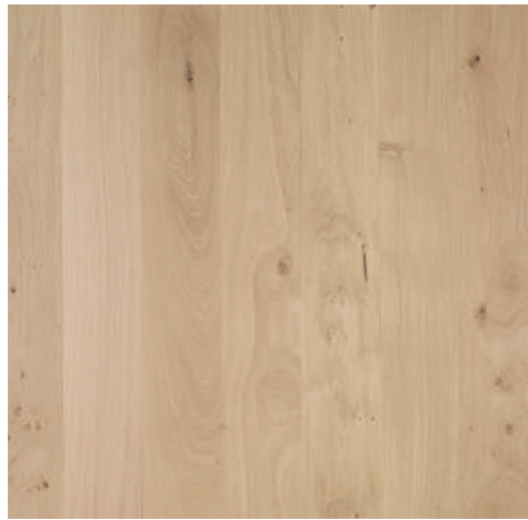
Authentic (Middle grade): light and dark wood, black knots, filled knots, partially opened knots, discolouration, black marks, cracks. The size of the knots is proportional to the width of the planks.
